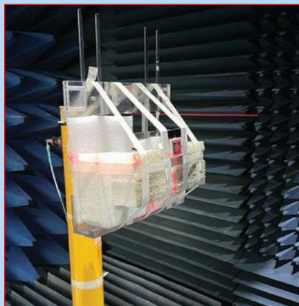
▲ Fig. 3 Anechoic chamber test setup.
