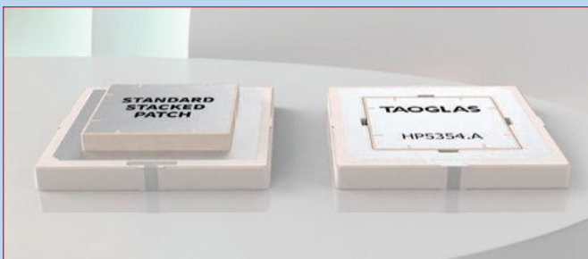
Fig. 1 Standard stacked patch antenna compared to the Taoglas Inception HP5354.A.
